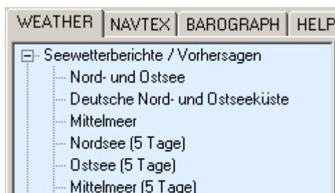
In order to view weather-messages please activate the tab WEATHER. Afterwards you can click on a message type in the weather menu structure. The appropriate message appears in the message window on the right side. The last two messages of each message type are indicated.
