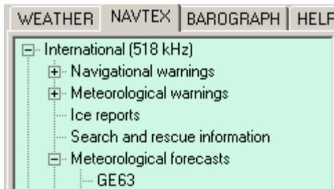
In order to view NAVTEX- messages, please activate the tab NAVTEX. Here the NAVTEX menu structure is shown, in which the NAVTEX messages are sorted according to their message type. For the two NAVTEX frequencies 490 kHz and 518 kHz two menu structures are available, one for each. The
