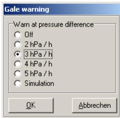
With fast changes of air pressure the gale danger is particularly high. In order to relieve you from the constant observation of the air pressure process, you can switch on the storm-warning. This function will be opened by the menu *Settings->Gale warning*.
