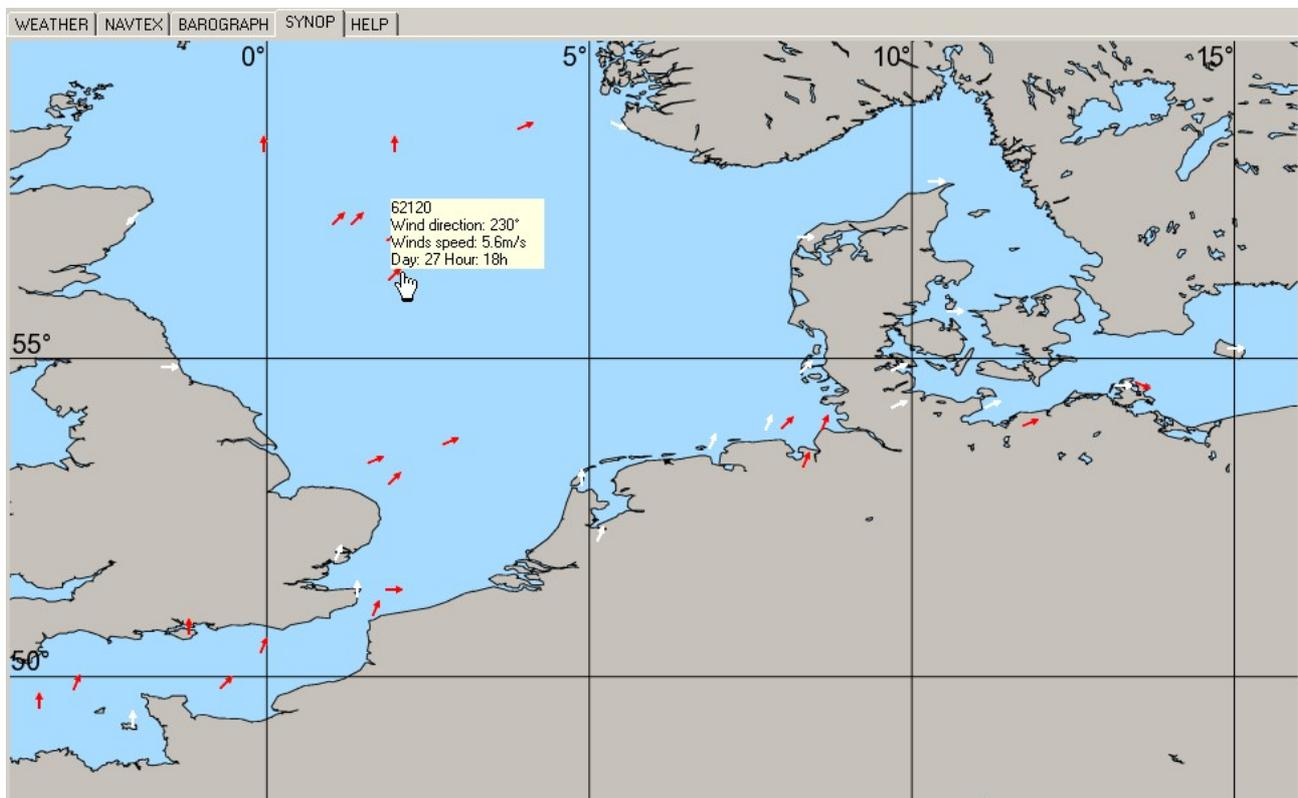
The WIB3-Software decodes these data and indicates it in a map as wind arrows.
