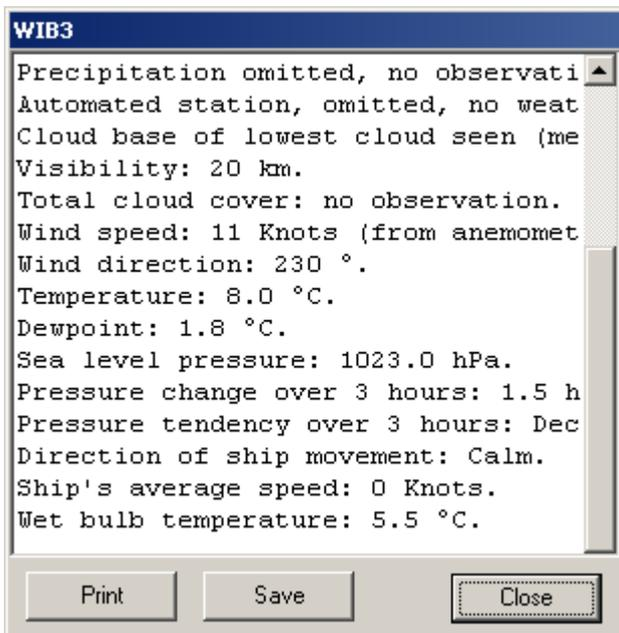
To display all decoded information of a Synop Message please click on the appropriate wind arrow (see page 9). A window will be opened with the data in plain text. If you click on a white arrow, the station messages of North / Baltic Sea are indicated. The station belonging to the arrow is marked by a star (\*) in the beginning of the line.
