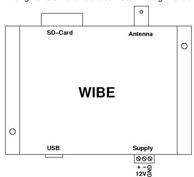
The antenna socket (BNC) can be connected with an active antenna (12V) or a passive antenna (e.g., isolated backstay with passivbalun).
