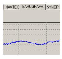
The fourth tab contains the BAROGRAPH. The measuring data are represented in the diagram from left to right. I.e. the current measured value is located on the right side of the curve. The barograph has a measuring interval of one minute and resolution of 0,1hPa.
